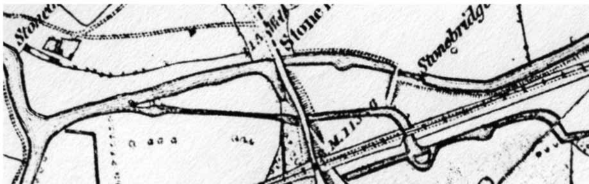
Wey and Arun Canal at Stonebridge – Showing the re-alignment of Cranleigh Water resulting from the construction of the Railway
